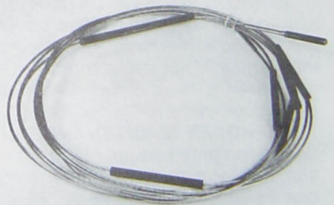
Typical wire headstay with marine eye and swage stud showing connectors, top foil trim cap and special top connector strung on wire.
