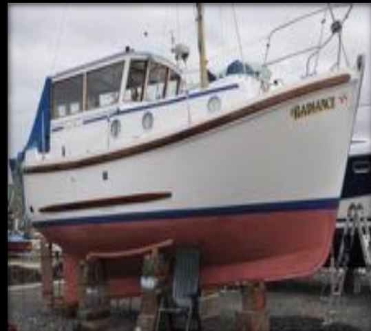
This CW is chocked correct, 'waterline' to earth
