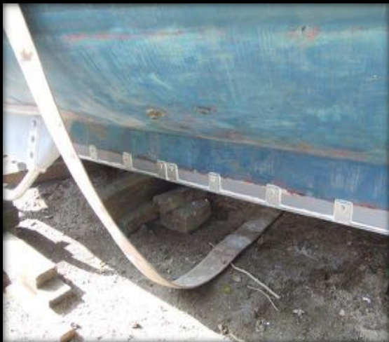
A good 10mm thick galvanised heavy 'Keel shoe' on a CW 28'-6"
