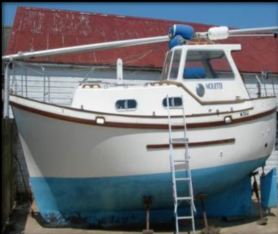
This CW is chocked wrong 'keel' to earth
