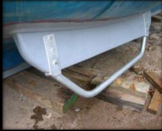
60mm dia tubular bilge keels on a CW 28'-6"
