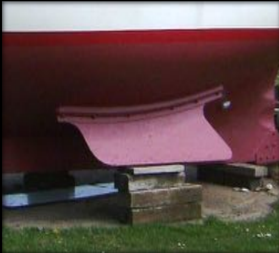
Shaped heavy duty bilge keels on a CW 28'-6"
