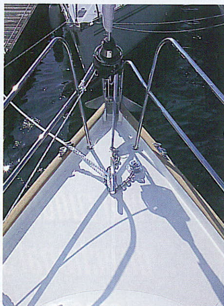
With no anchor well and a single, central cleat, the foredeck is uncluttered
