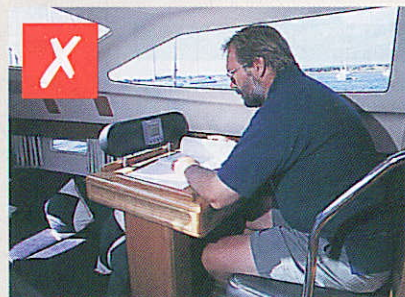
Chart table with a view – but where do the plotter or radar displays go?
