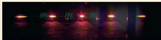
A typical diffraction pattern from a red LED navigation light
