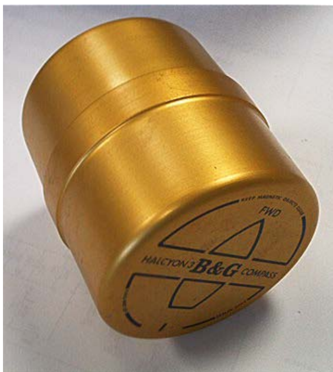
Sensor viewed from the top showing mounting orientation
