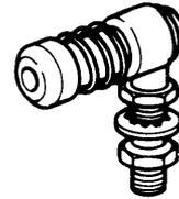
A31126-Quick-release type, the stud is 9/16" long with 1/4" 28 UNF threads. 15/16" from center of stud to end of barrel. Complete with nut and lock washer.
