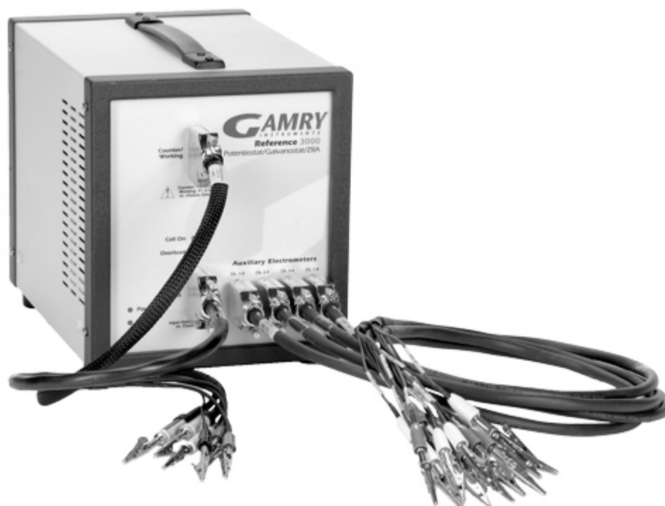
Figure 5.5 GAMRY Reference 3000 potentiostat [79].
