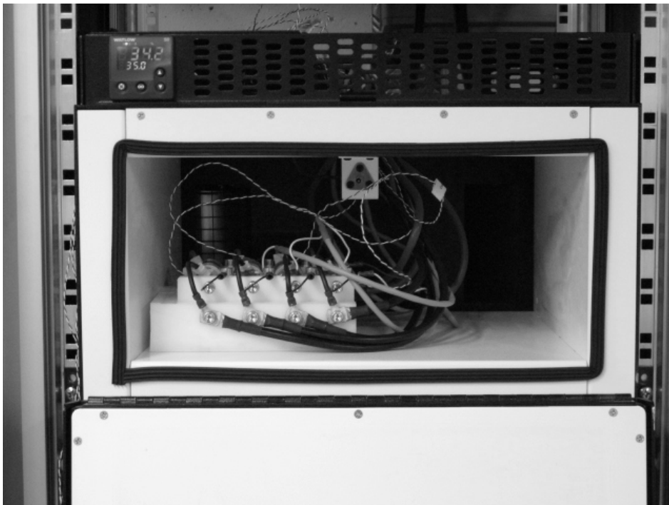
Figure 5.7 Maccor climate chamber with cell fixture.
