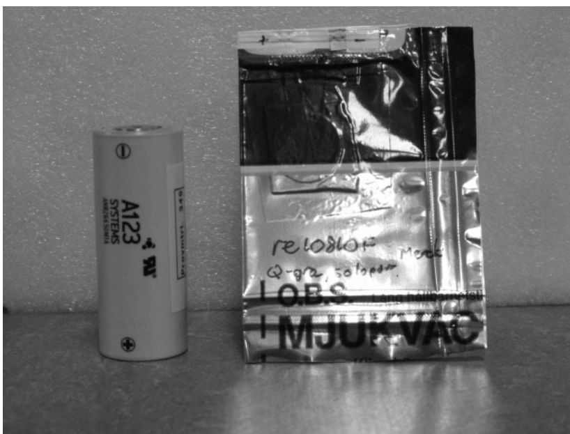
Figure 5.3 A123ANR26650 cell and 3 mAh half-cell from UU.
