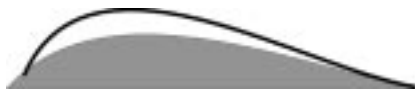
Shaded portion represents sail with tight headstay. Unshaded shows increased depth as headstay sags.
