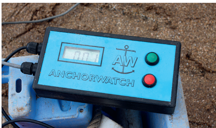
Anchor loads are measured using the Anchorwatch system
