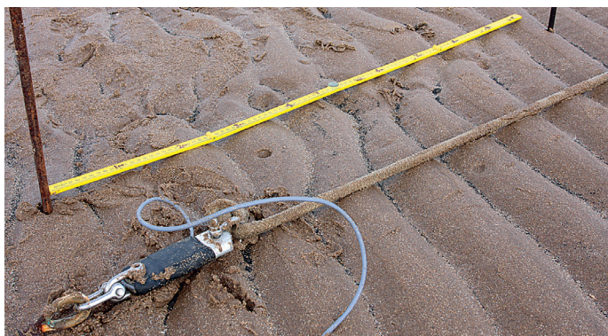
The distance dragged is measured at the shackle of the load cell
