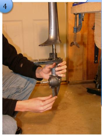
4. One of the major causes of outboard failure is due to overheating. Many owners do not realise that the engine has a water pump and this often goes ignored. I like to check the impeller every year and replace it as a matter of course.
