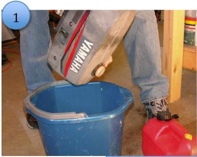
1. After running the engine to engine to flush the water ways through with fresh water empty out all the remaining fuel. If the engine is large you will have to
