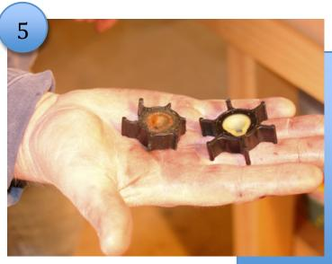
5. No prizes for guessing which is the new impellor. The old one on the left had only to blades left and was long overdue for replacement, and had been causing chronic overheating problems with the engine, which was no surprise. Try to find the missing vanes if you can as they often get trapped in the outflow from the water pump restricting the flow of water up the leg to the engine. A blast of air from a compressor often blows them
