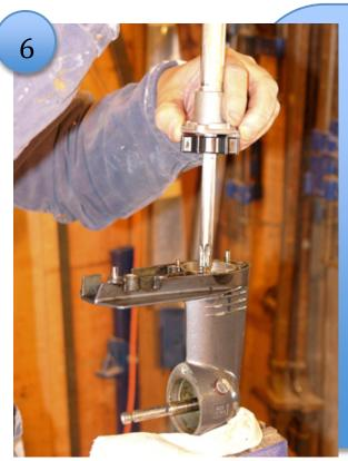
6. Slide the water pump top housing and impellor onto the drive shaft and reinsert this back into place. Don't forget a new gasket between the two halves of the pump.
