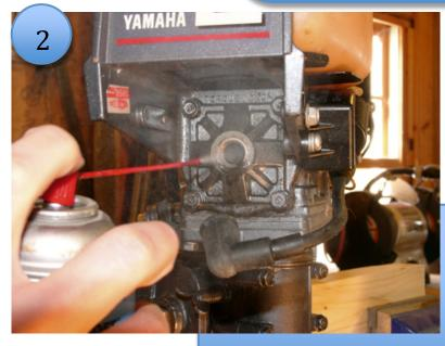
2. Remove the spark plug or plugs and spray in some fogging oil. Pull the start cord a few times to coat the interior of the cylinders then replace the plugs
