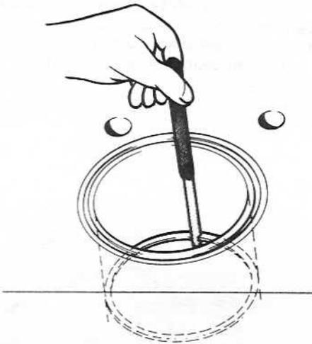
22. Insert a new piston ring into the cylinder and measure the piston ring gap. As to the measurement, see under "Technical Data". If necessary increase the gap, using a special file.
