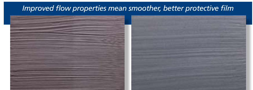
A competitor's epoxy primer. The thickness of the paint is uneven due to its poor flow characteristics. As a consequence the recommended film thickness may not have been achieved in the 'valleys' between the brush marks.
