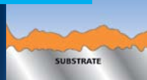
After first primer coat film thickness is too low in places.
