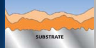
Second primer coat fails to achieve required film thickness in places – trouble ahead!
