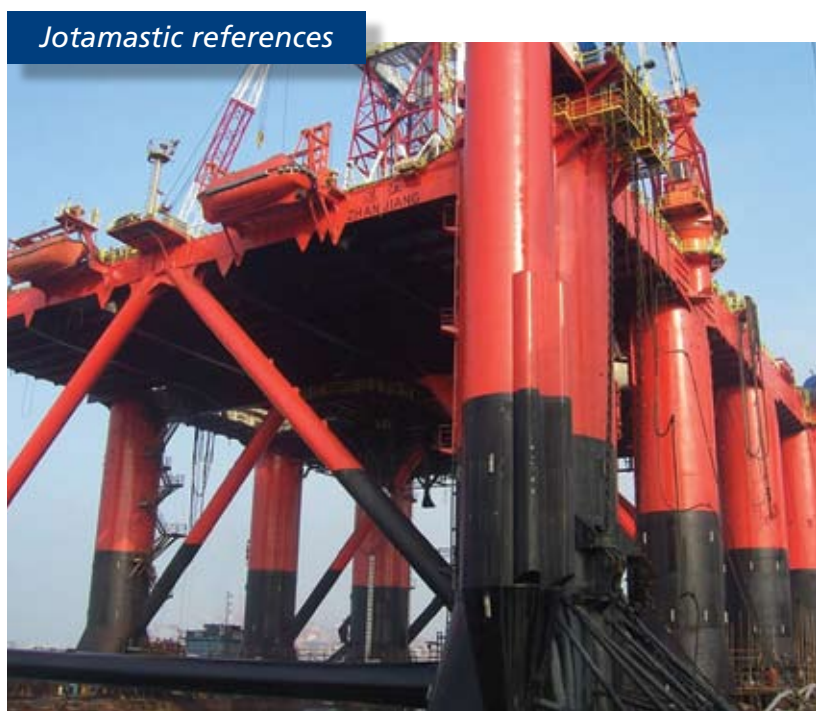
Above: Nanhai 2 semi-submersible rig Drydocked at YouLian Shipyard in China and was protected with Jotamastic GF and a topcoat of Hardtop AS.
