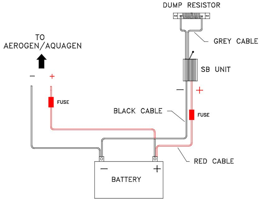
SINGLE BATTERY VOLTAGE REGULATOR WIRING DIAGRAM
