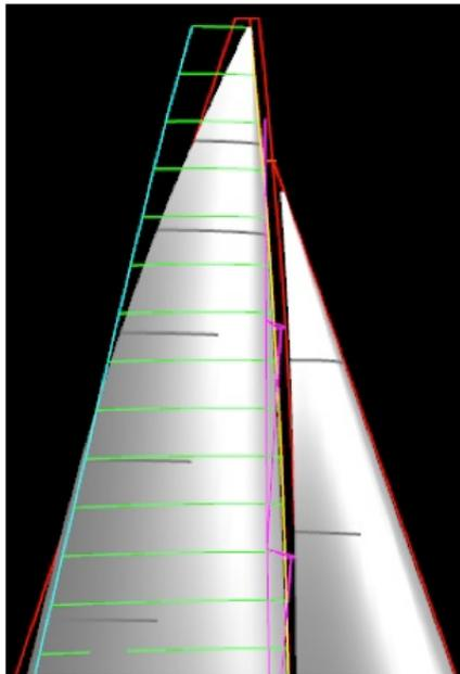
**A moderate square-top main (light blue outline) can provide extra horsepower and a better twist profile, all for a relatively modest rating increase.**
