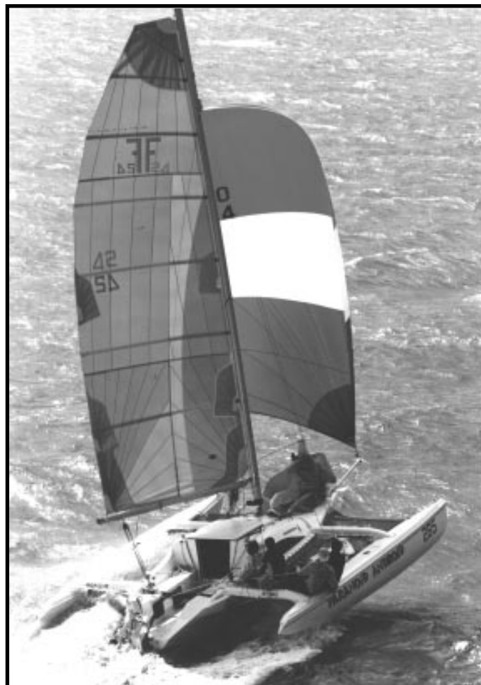
Asymmetric spinnaker on an F-24 Mk II being raced very hard. Note the extra long tiller extensions each side rigged up by these Australian skiff sailors, which are held in place by shockcord to the aft beams. Works very well.
