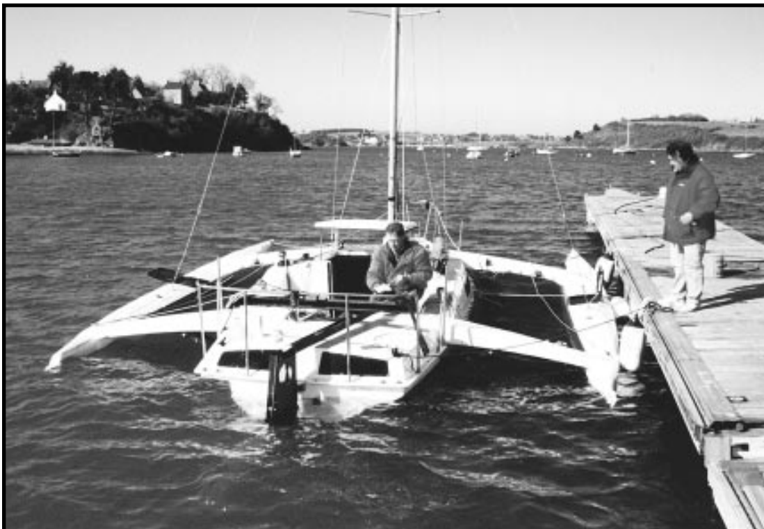
Even when fully flooded, a Corsair will stay afloat easily. This F-27 was deliberately flooded in order to demonstrate its unsinkability.
