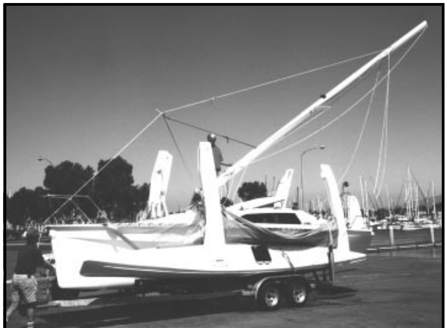
Mast on its way up and being held from going sideways by raising wires
