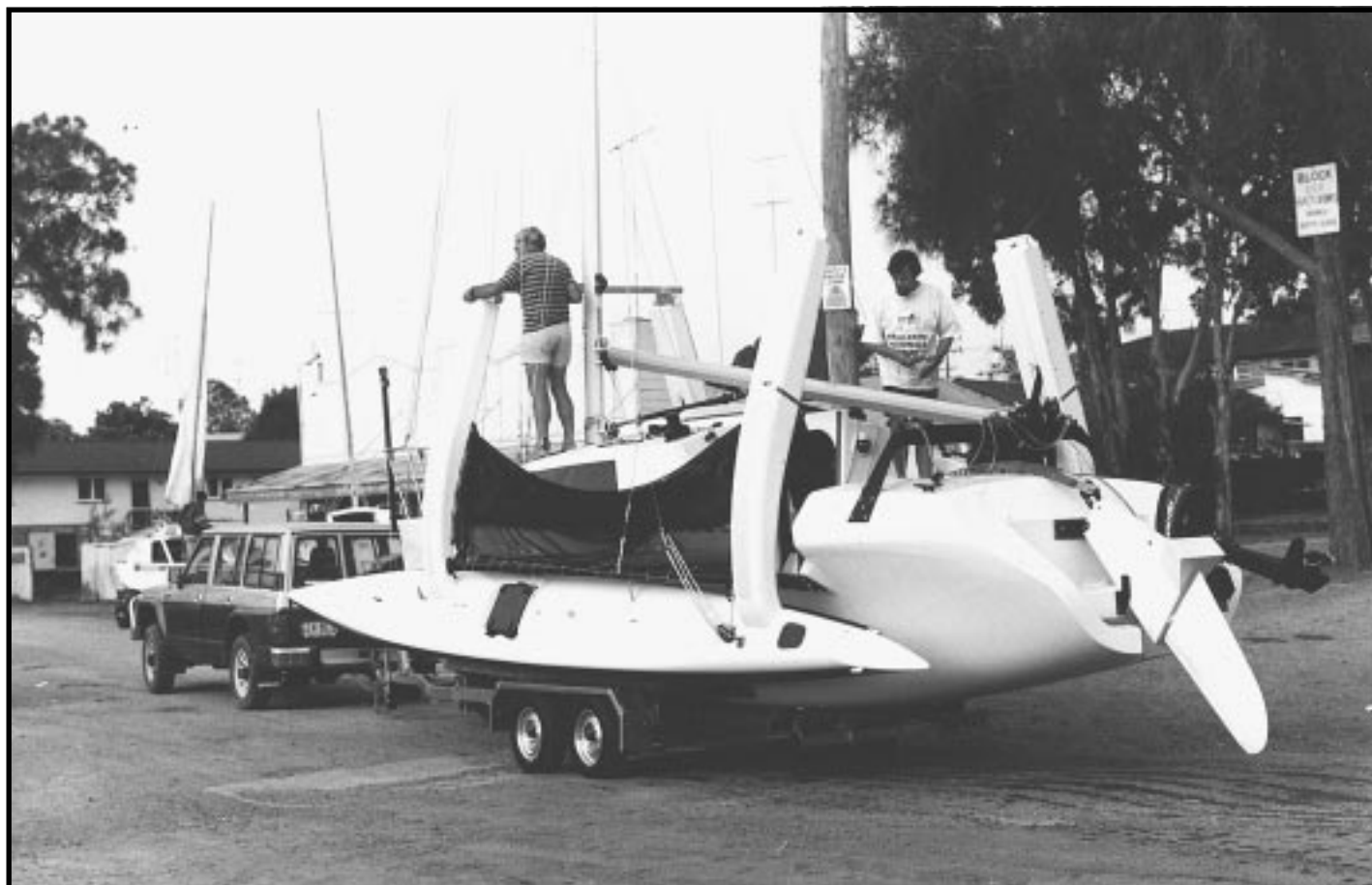
The original prototype F-31 aft cabin, with outboard and underslung rudder system. This type of rudder can be removed altogether for long distance trailering. Aft cockpit models all now use transom hung rudders.
