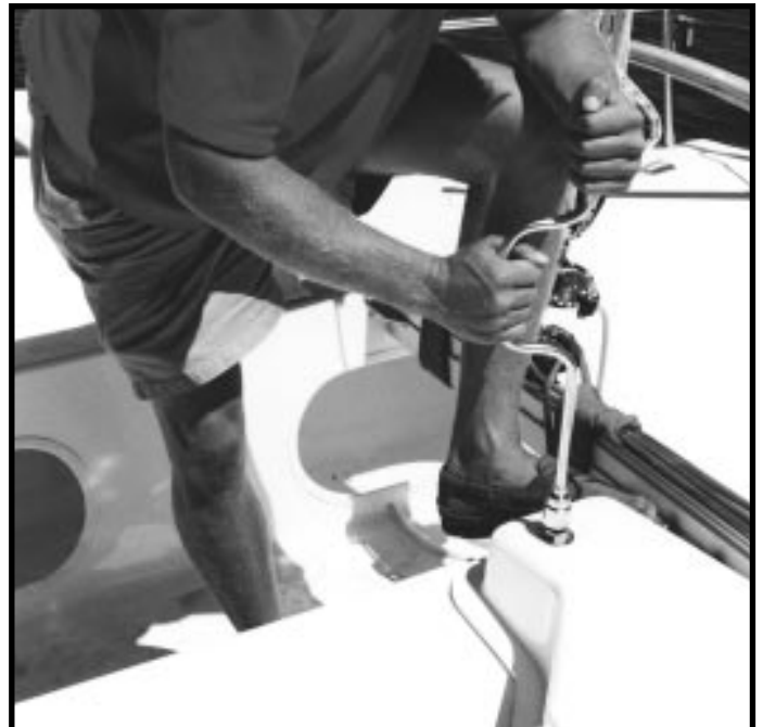
Beam bolts must always be tightened firmly before sailing
