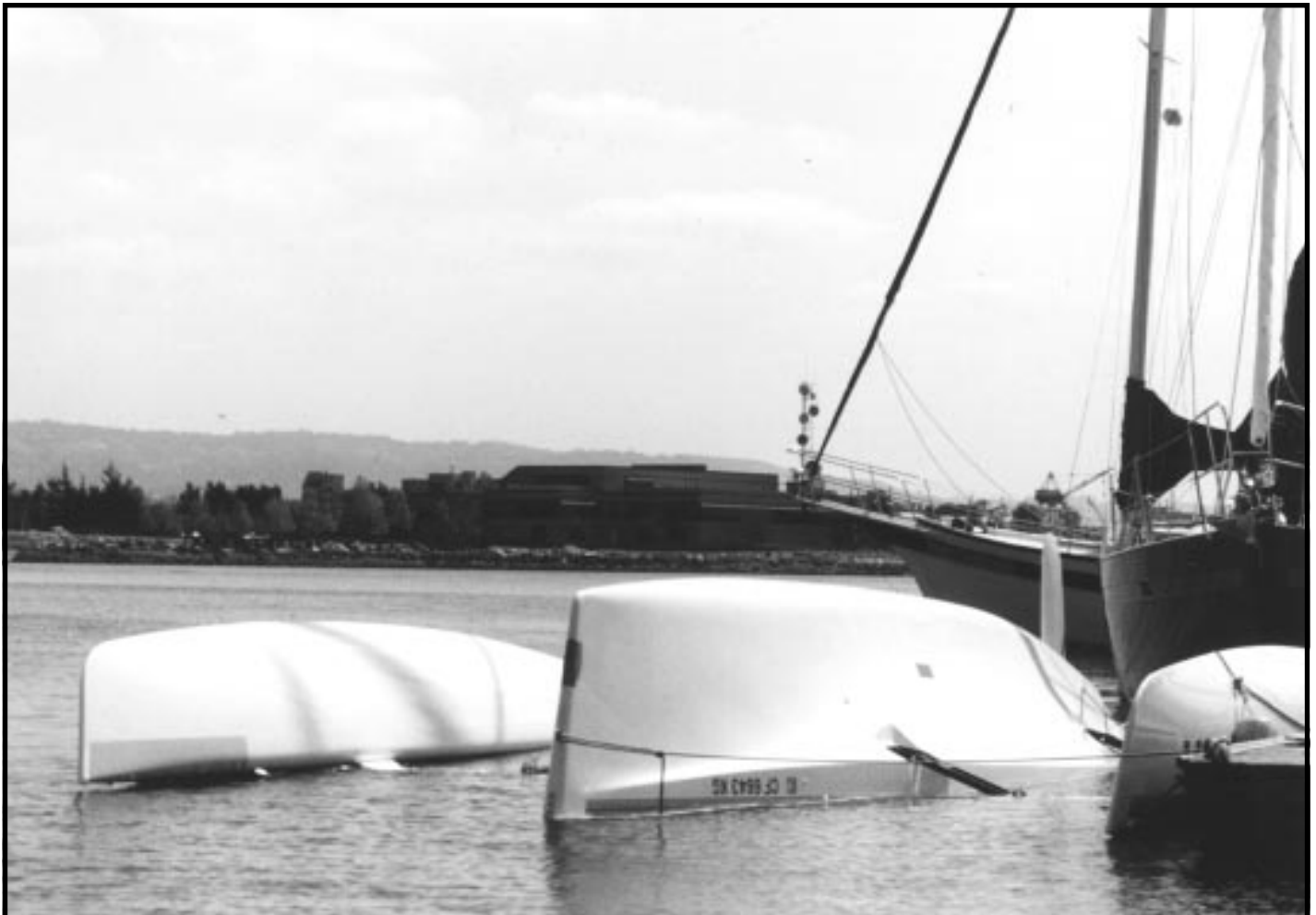
Push it too far and this is what may happen - a capsized F-27 - note how high it is floating, the water level being around the bottom of the beams. Even in this position it remains a relatively easy and safe boat to move around on.
