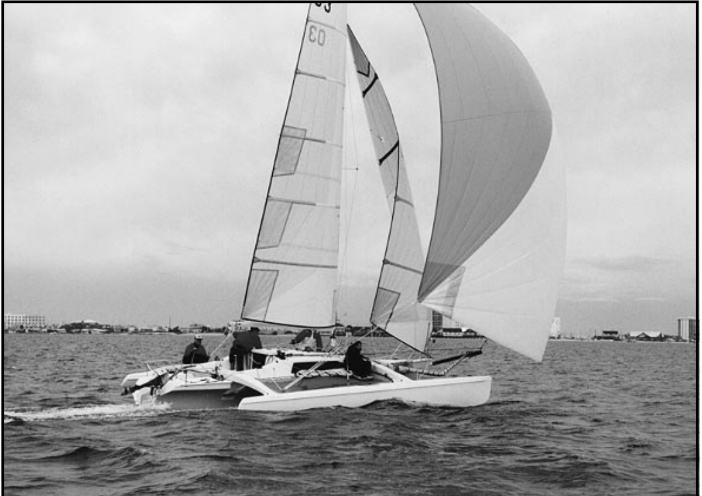
Asymmetric spinnaker on an F-28R. Jib can be flown inside by racers as shown for better performance in light airs
