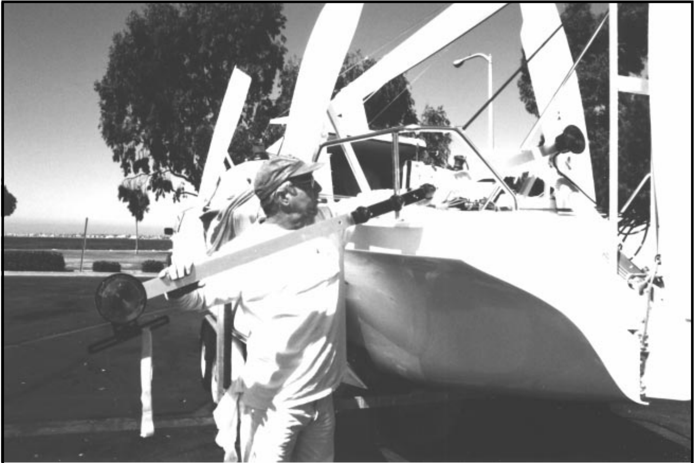
Light bar being fitted on an F-28. Note vertical position of transom hung rudder blade for trailering
