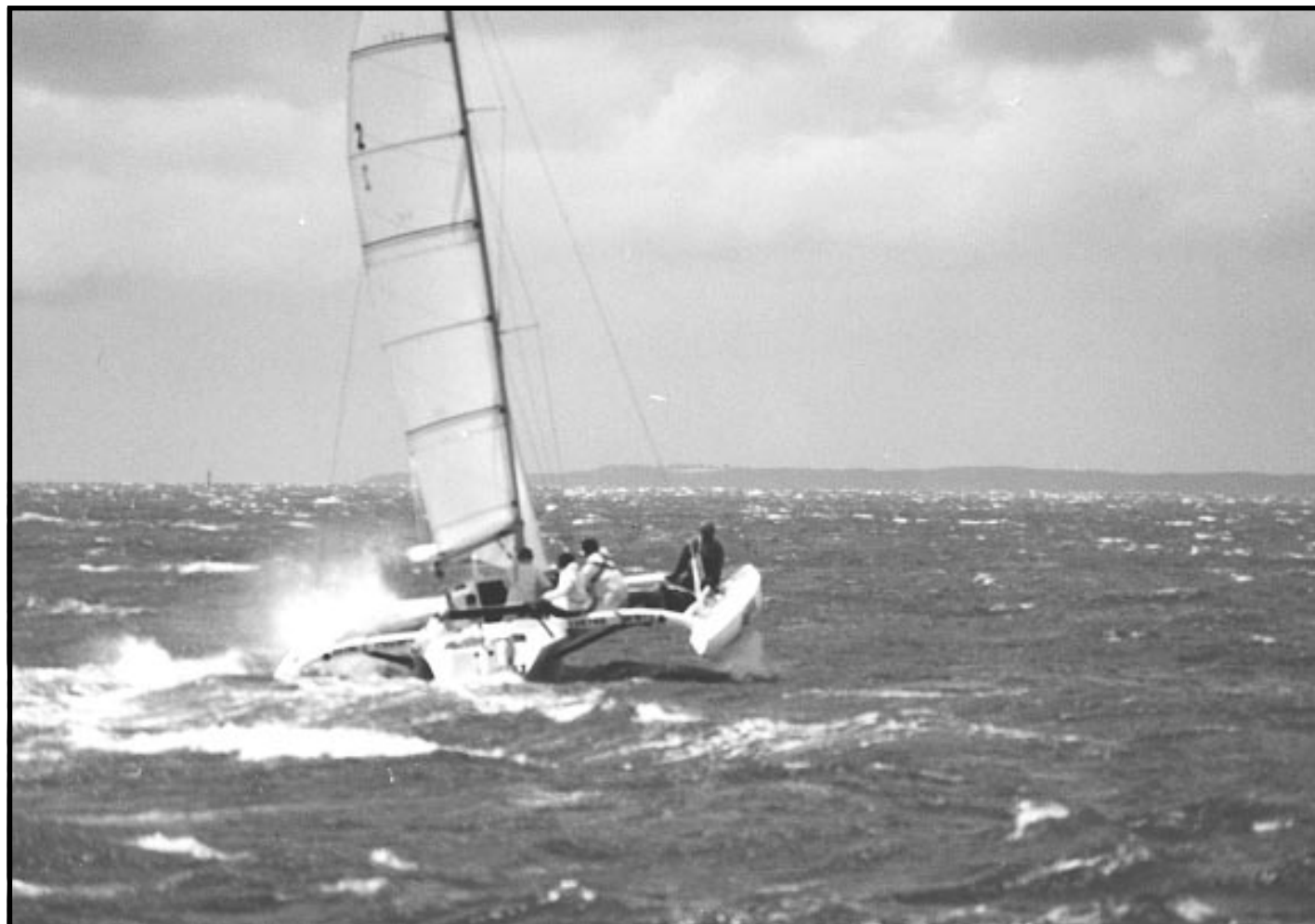
Set up and sailed properly, a Farrier design is a very safe, yet very fast boat. This F-31 is powering into 25 to 30 knot winds, with a single reef. Speeds of around 11 knots to windward are possible in such conditions
