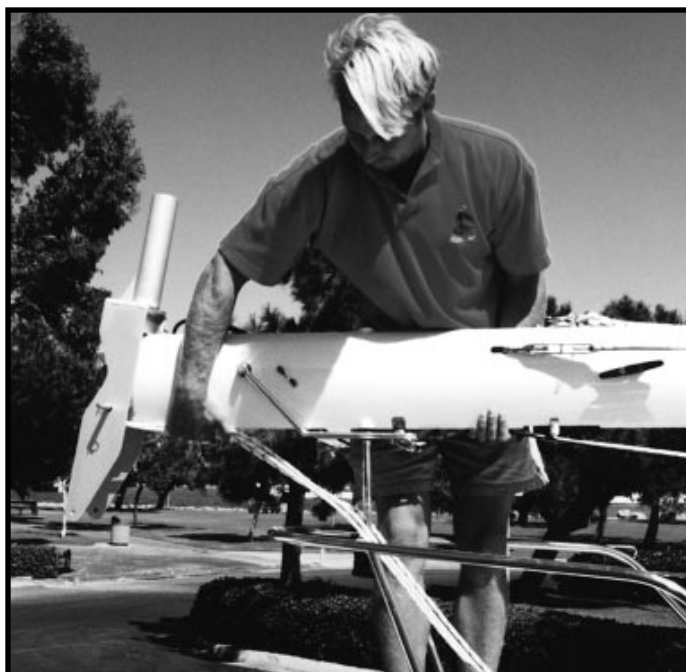
Fitting an F-28 Mast to pulpit. All such masts with roller furling fit on a vertical 'swing up' spigot on the pulpit. Mast raising pole yoke can be left on mast as shown if wished. Note also rotator position - folded up against mast.
