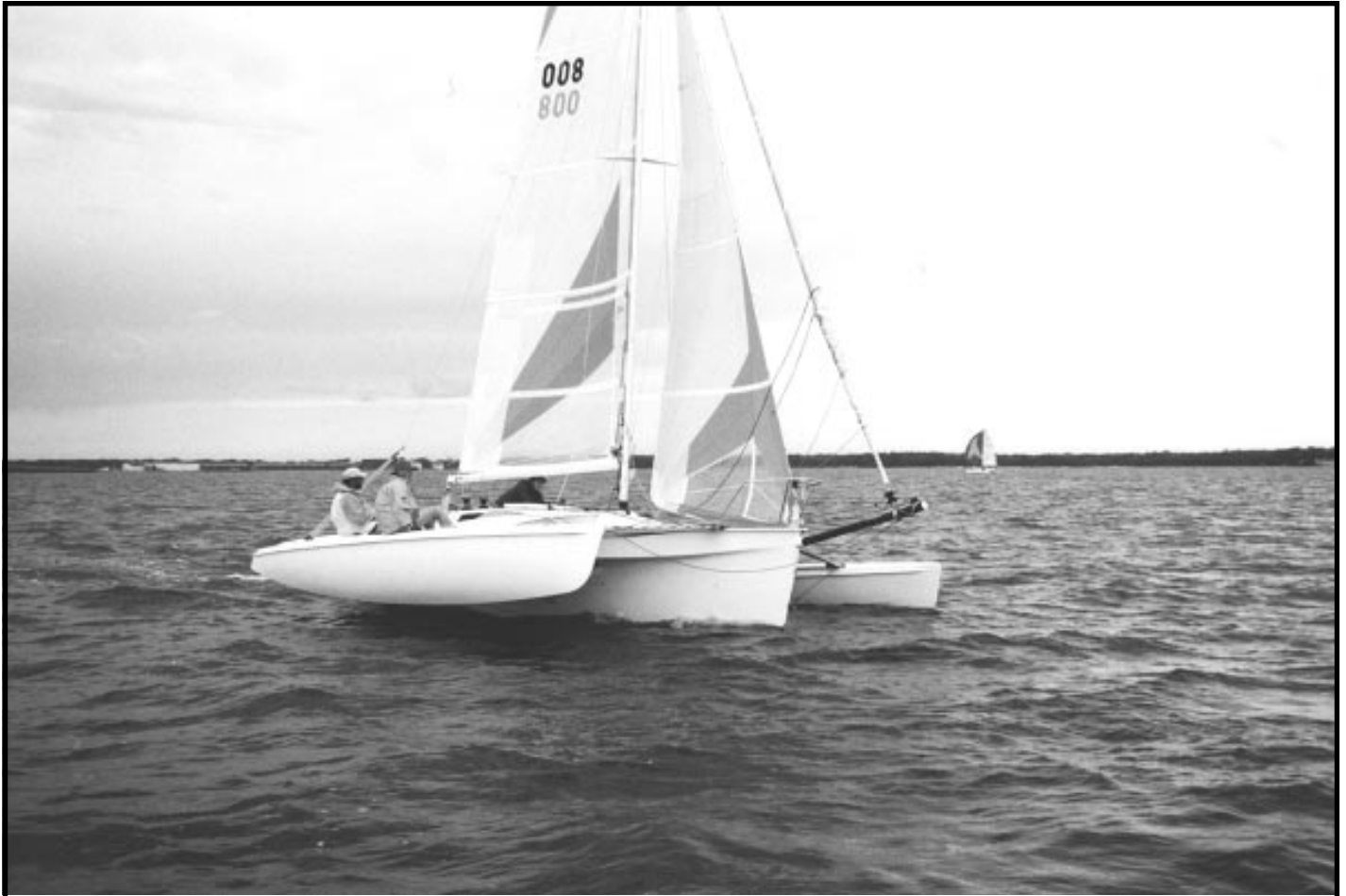
Achieving good windward performance can be very satisfying, but it does depend on a lot of factors being right. Screacher can be left up permanently as shown on this F-28R
