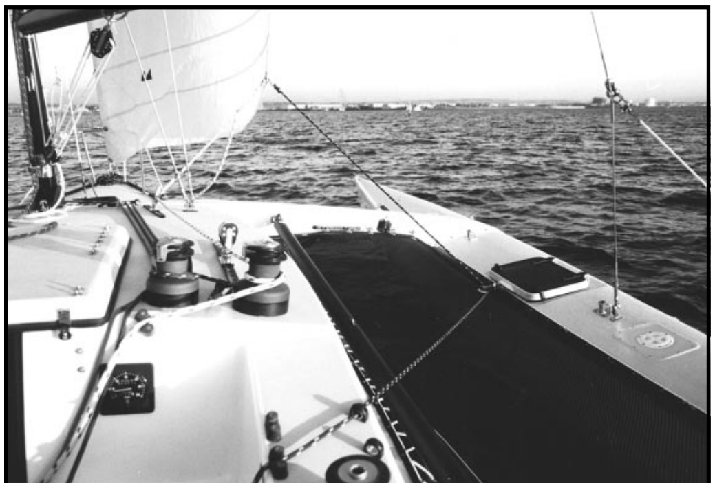
Jib barber hauler in use on an F-27 - will considerably boost performance
