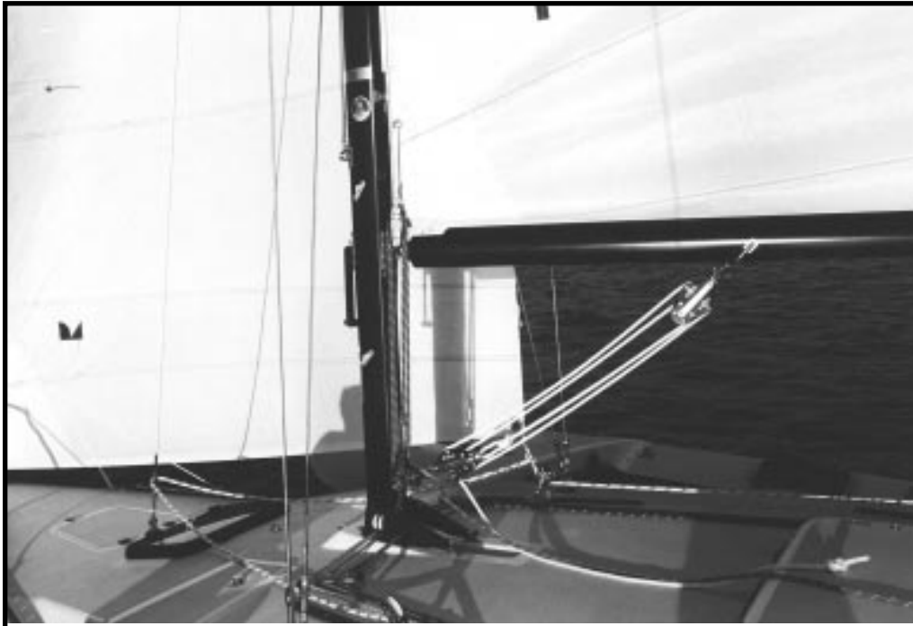
Boom vang and Cunningham eye controls on an F-27
