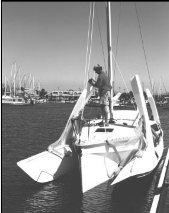
Unfolding can be done at the dock or while motoring away. But beware, while folding stability is good, it is limited.
