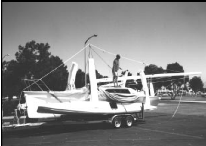
Mast raising pole in position on an F-28 with winch line connected to jib halyard, ready to raise mast. Shrouds must be attached to floats to prevent mast falling forwards.
