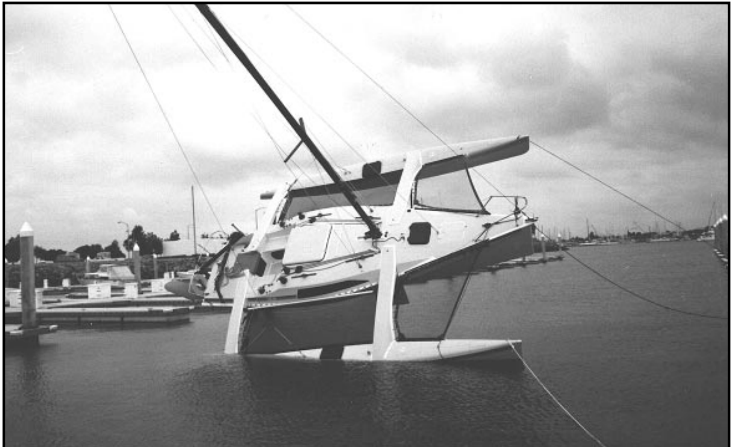
This is not a safe angle of heel - go this far and you are probably gone! This F-27 is being pulled over to test stability.
