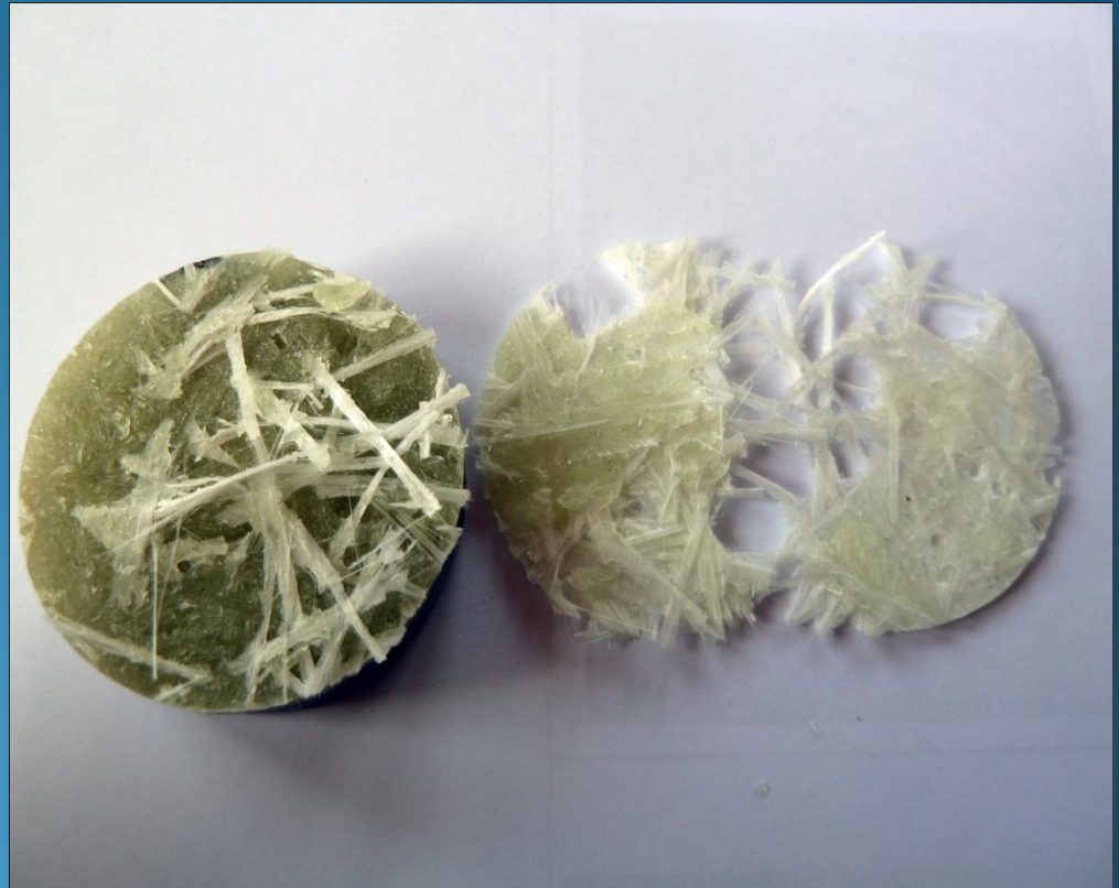
Drill Plug no 3. Parts that came out during the tensile test..
