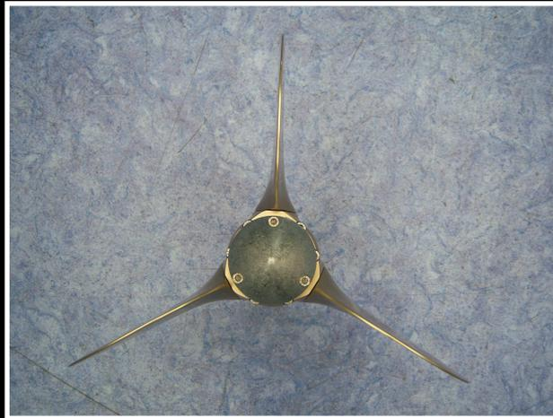
DANS LA POSITION EN DRAPEAU, LES PALES DOIVENT ÊTRE PARFAITEMENT ALIGNÉES SUR L'AXE DU MOYEU (VOIR PHOTO CI-CONTRE).
