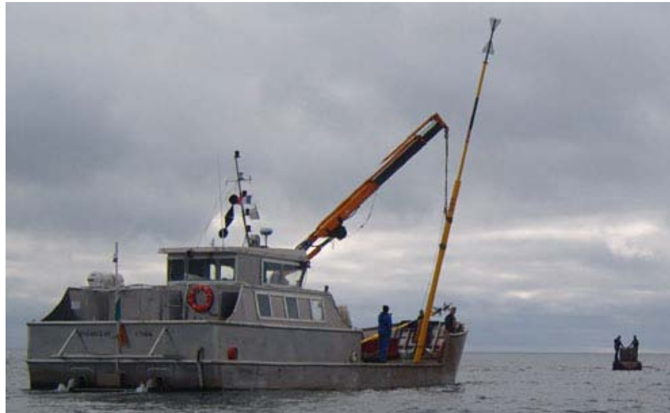
Assistance Phares & Balises : pose de la balise renforcée du "Trehu" à Groix : diam 160 - 1,6 tonne. Assistance to the Lighthouses department, in very shallow waters.
