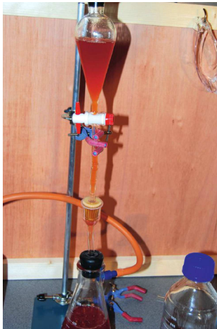
We filtered 500ml of treated fuel through a 10 micron filter
