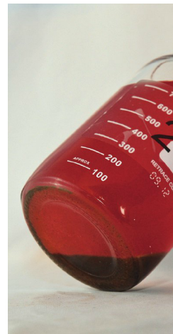
Deposits and poor dispersal suggest inadequate dosing
