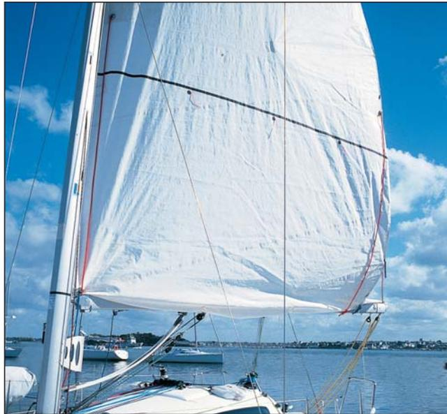
This automatic reefing system is the ideal solution for reducing sails easily and avoiding friction on grommets. Combined with a set of deck blocks in the boom, you can directly take in reefs from the cockpit.
