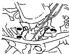
THROTTLE CABLE AND PIVOT SHIFT SHAFT AND PIVOT
