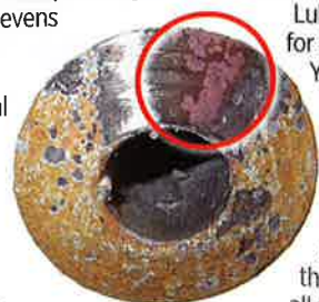
Pink spots on this 2009 Elan seacock are an obvious sign of dezincification
