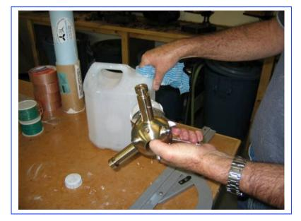
**EXAMPLE:** Pre loading the torsion spring on a **RIGHT HANDED** propeller unit:
