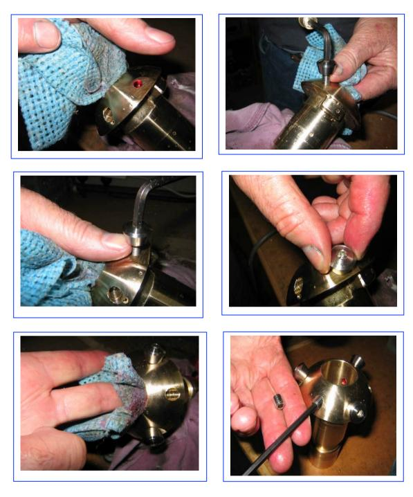
TORQUE TO 18 Nm (24 ft lbs) with a TORQUE WRENCH - DO NOT TIGHTEN WITHOUT A TORQUE WRENCH CHECK THE CONTACT SURFACES WITH THE BLADE CARRIER VERY CAREFULLY TO ENSURE NO BURRS REMOVE WITH A FINE RIFFLER FILE IF REQUIRED.
