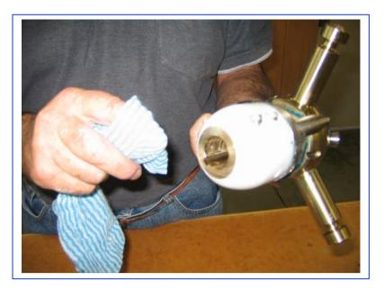
**FINALLY: SEAL** the grooves in the Nose with 3M 5200 and the exist holes of the Screws on the Nose
