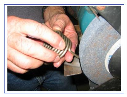
Grind and bevel both ends of the torsion spring to ensure that it slides easily into the Acetal Nose cone. Any sharp edges will bind during final assembly
