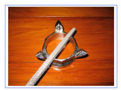
Check the inner corner of the Tripod to ensure nothing protrudes that could impact upon a flush fit against the blade carrier
