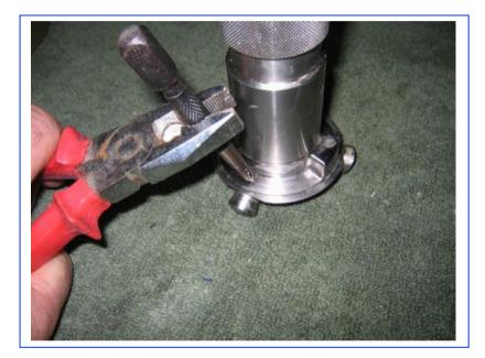
Mount the Boss as shown to expose the sections where the Reverse Rollers are approaching the internal surface of the Boss.
