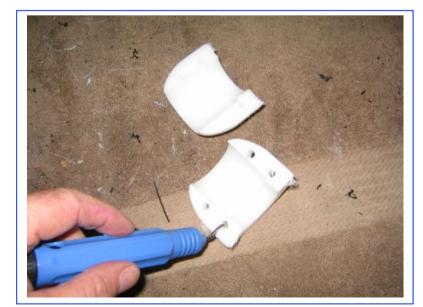
De-burr all the cut surfaces using a deburring tool. Include the 8 x holes and front internal diameter which was cut off on the lathe
