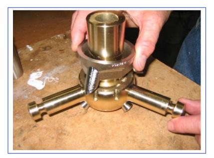
Mount the tripod into the grooves as shown for a Left Handed unit.
