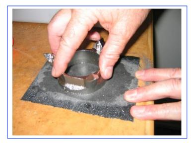
Sand on wet and dry or emery paper to remove any burrs on the face from any tearing of the SS which has left other than a very smooth surface.
