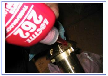
Smear a small coating of grease into the reverse roller surfaces that interface with the screw. This will prevent the Loctite™ causing the reverse rollers to bind together later
