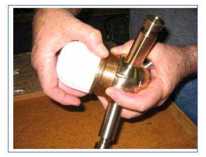
Expand the jig by rotating the two components in each hand so as to undo the threaded portion of the jig and eliminate all clearances between the components.
