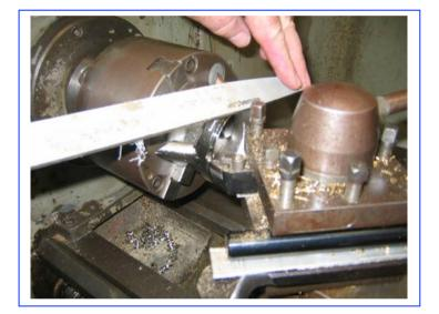
Remove aris from outer edge while Lathe is running with file
