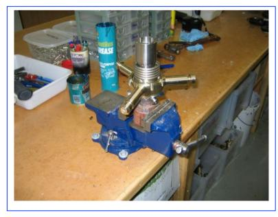
Mount the Boss over the wooden spigot as shown with the Blade Carrier in the correct registration. See Above.
