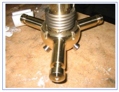
Check that the spring goes down the hole so that the first coil lies flat against the Blade Carrier, This requires that the fairing section above the hole is correctly positioned.
