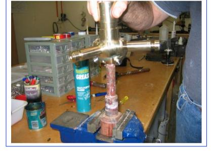
WIPE THE BOSS CLEAN BEFORE INSERTING SPRING
