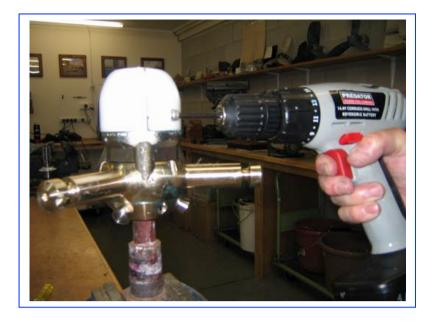
Place a small portion of 3M 5200 on the ends of each of the 4 Socket Head screws
