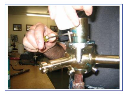
After ensuring the boss surface is clean – hold the spring tail out with a screw driver and mount the lower half of the Nose Cone onto the boss
