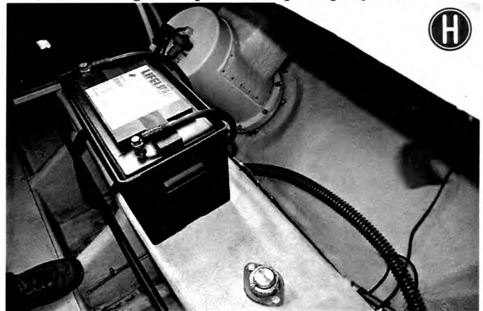
H: The location for the driver unit is just as important as the transducer. It must be one which can NEVER interfere with any boat operation and one which won't be stepped on if you need to get into the area.
