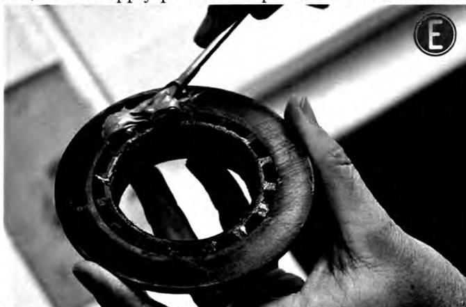
E: Apply a good layer of mixed glue all over the roughened base of the flange, again making sure you don't get any on the thread. You have quite a while before it starts to cure so take your time!
