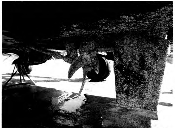
Same boat, eighteen months after cleaning AND having the original SILICON CHIP ultrasonic anti-fouling unit fitted. This illustrates that boats still need to be taken out of the water periodically but it's a whole lot better than the shot at left!
