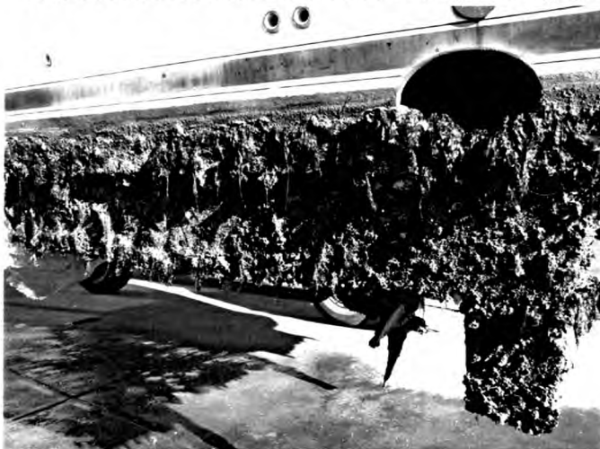
Excessive fouling after a boat had been in the water for two years with minimal usage. There was no Ultrasonic Anti-Fouling fitted. This amount of growth would severely impact speed, handling and fuel use.
