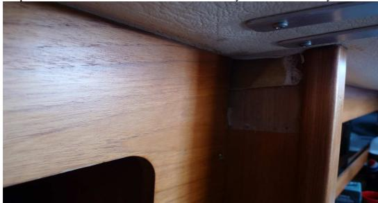
6. Remove the wooden cover plugs from both the top and bottom panels and ensure that the screws will move. ( I had to drill one out )
