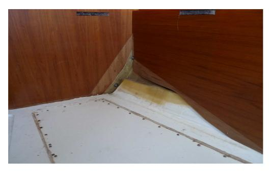
4. Remove trim panel on the top forward bulkhead near the window by sliding sharp blade between it and the bulkhead and carefully lever it off—held by 3 small tacks
