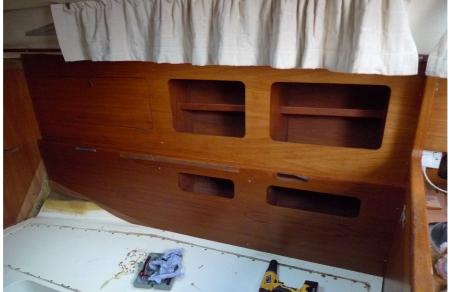
7. Remove the screws from the bottom panel and then carefully slide it out – forward end first – supporting the weight of the top panel.
