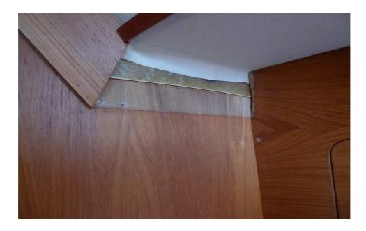
5. Remove trim panel on the top of the bulkhead next to the galley near the window by sliding sharp blade between it and the bulkhead and carefully lever it off—held by 3 small tacks
