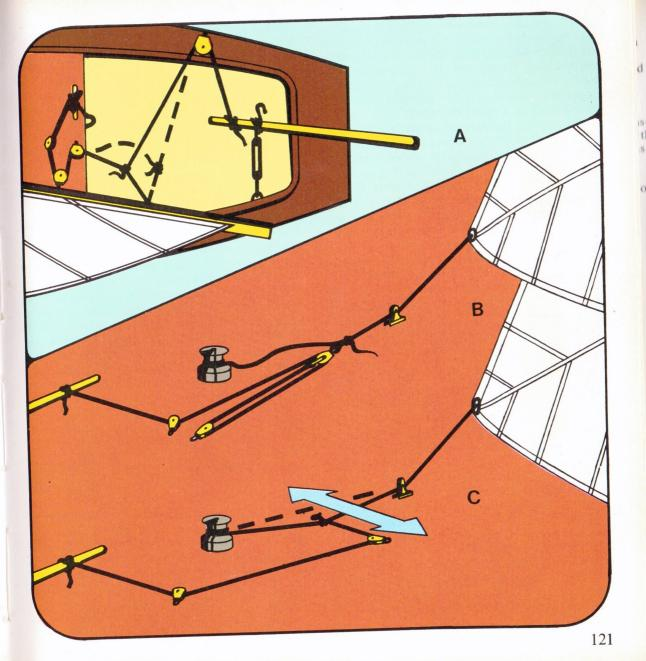
show how a tiller line can be attached to a sheet so that only a part of the sheet's pull is used to steer the boat. If a special tiller line like this is used the self-steering system can be disconnected immediately without touching the sails, and this is an important safety factor, for example if the boat finds herself on a collision course.
