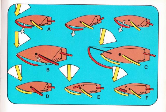
8.7. There are various ways of getting the boat to steer herself when the wind is abaft the beam. The most practicable methods are amongst those shown here and in every case the sheet is made fast to the windward side of the tiller.
