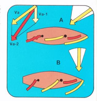
8.6. Sails steering the boat when the wind is forward of the beam. The arrows indicate the wind direction that matches the way the sails are trimmed in the sketches, while the arcs show the range of wind direction through which the relevant systems can be used. To keep the sketches as simple as possible the sheet is shown leading direct to the tiller, although this is less likely in practice.
