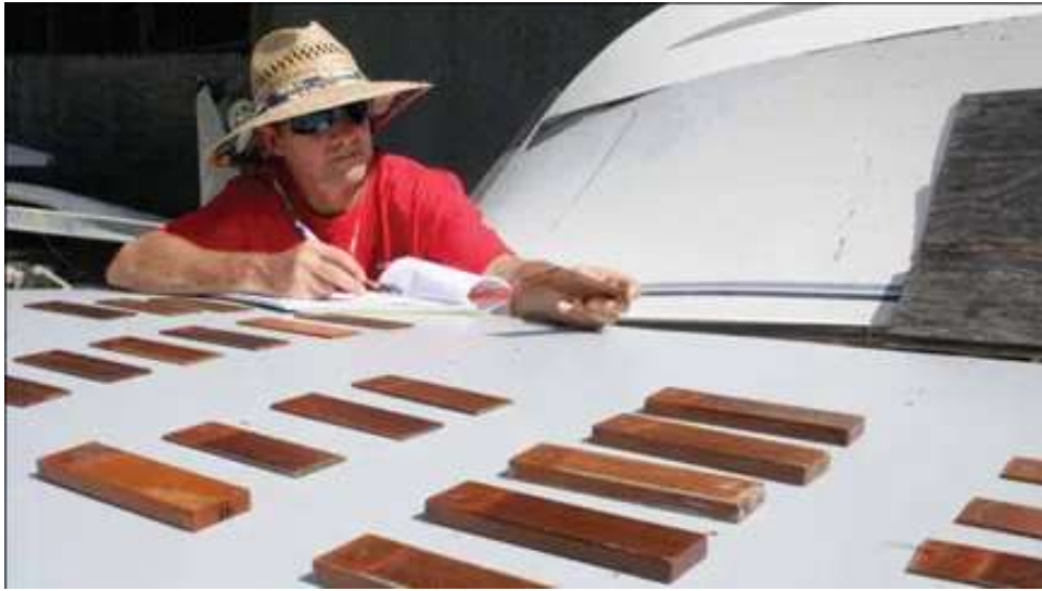
After two years of testing, its apparent that two-part varnishes are the most durable type of exterior wood finish.
