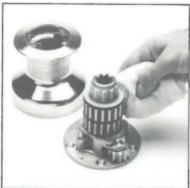
Wash centre stem, roller bearings and drum bore with kerosene (paraffin). Dry with a non-fluffy cloth.
