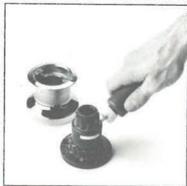
Lightly grease centre stem.
