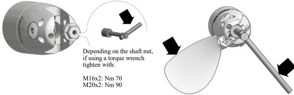
**2** Slide tab washer (5) onto the shaft nut locking screw (6). Attempt to position the tab relative to a flat side of the nut. Insert the screw (6) through the hole in the shaft nut. Tighten the screw firmly into the end of the shaft. If using a torque wrench tighten with 15 Nm; (1,5 kpm, 10.8 ft-lb.)
