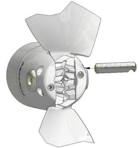
**7** Insert the last pivot pin locking screw (9); turn it to engage a couple of threads; It will be tightened in step 8.
