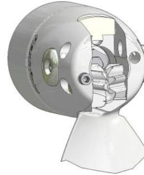
**6** Align the last blade (7) with the blade socket in the hub and insert a pivot pin (8) with the notch in pin aligned with the hole for the pivot pin locking screw. Move blade slightly to ease operation;
