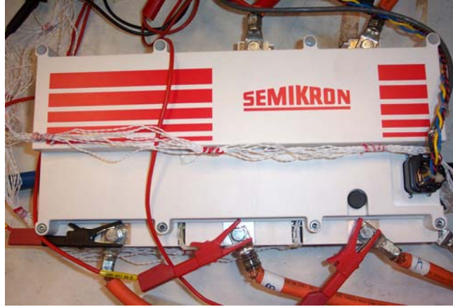
Figure 5. Semikron inverter unit.
