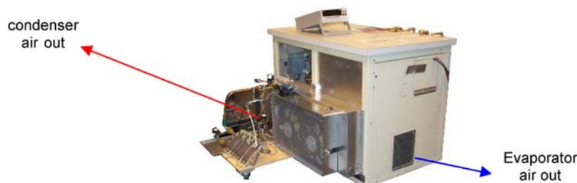
Figure 2. Revised floating loop attached to full-size sedan AC system in a cabinet.
