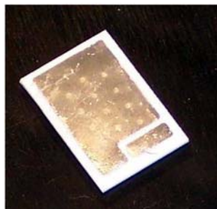
Figure 9. A two-side solderable die obtained from Rockwell Scientific.
