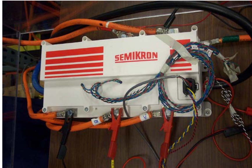
Figure 1. Top view of Semikron AIPM unit.
